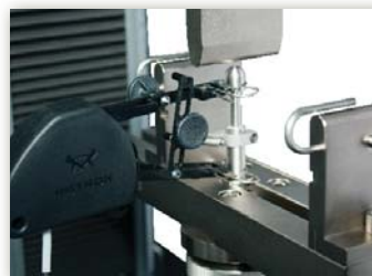
Deflectometer using Clip-On Extensometer
