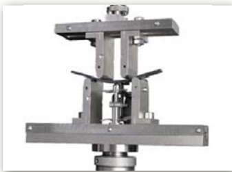
Four-Point Flexure Fixture using Midpoint Deflectometer
